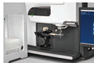
Advanced valve system 4-port switching valve (AVS 4) fitted to a 4210 MP-AES
