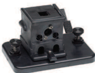
Thermostatable cell holder, 89054A
