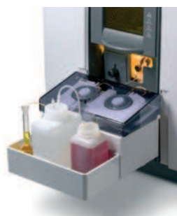
SIPS 20 Sample Introduction Pump System for flame AA
